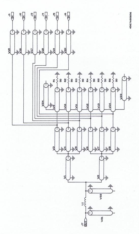
6:1 Combiner Assembly 1A1A1A1A3,1A1A2A1A3 - Electrical Diagram Figure 2-11.
