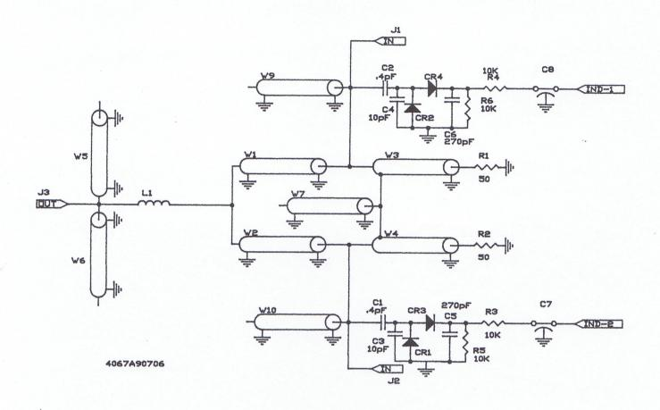
Figure 2-12. 2:1 Combiner Assembly 1A1A1A7, 1A1A2A1A3 - Electrical Diagram
