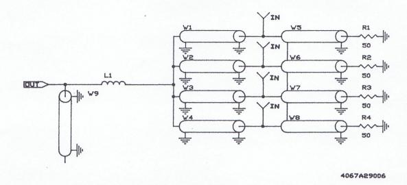
Figure 2-9. 4:1 Combiner Assembly 1AlAlAlAlA3,1AlA2A1A1A3 - Electrical Diagram
