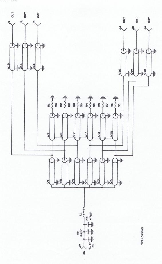
Figure 2-10. 1:6 Divider Assembly 1A1A1A1A2, 1A1A2A1A2, Electrical Diagram
