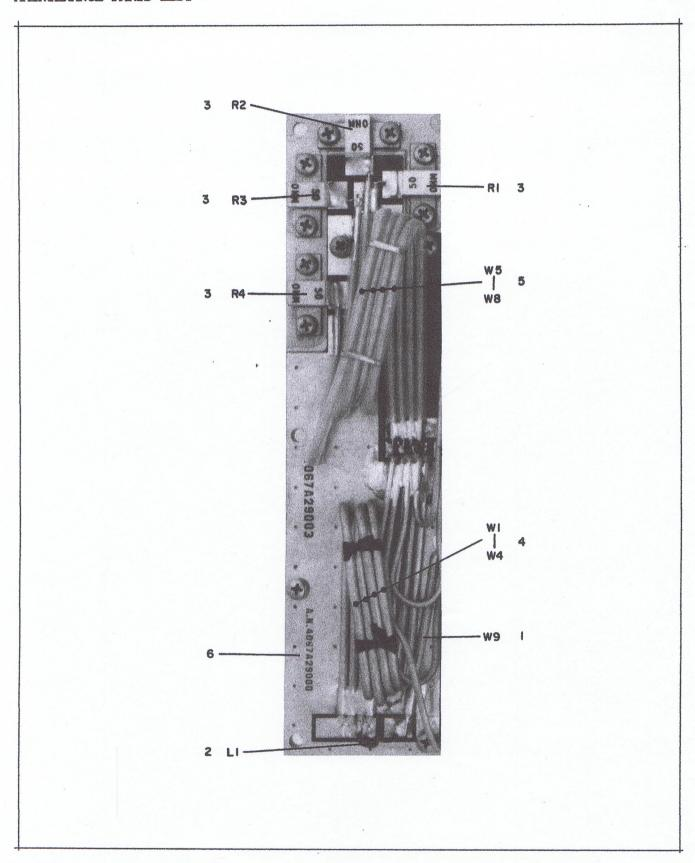
FIGURE 8. COMBINER ASSEMBLY, 4:1, 1A1A1A1A3, 1A1A2A1A1A3
