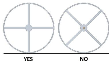
Rotors in casing, standing / or during maintenance in vertical position, should be secured so they can't fall. Rotor in casing can have a weight of up to 600 kg, an accident can cause serious health injury. Please store the rotors in a way so external damage impact is minimized. The rotor itself is quite fragile if hit by external impact.
