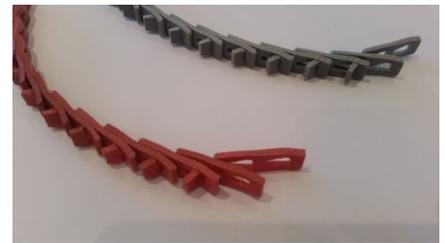
*\*All belts require adjustment, some once other a couple of times, depending on the environment they work in. Belt should be shorter than calculated length. When it comes to the power-belt, 1% is equal to 1 link per meter belt.*
