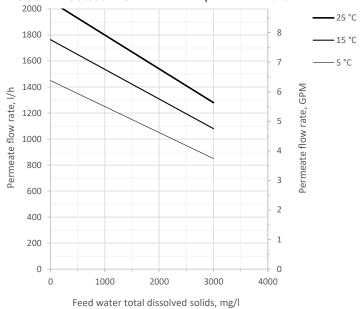
Permeate flow rates are calculated under the following conditions:
